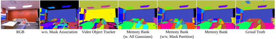
Fig. 10: Visual comparison of different mask association methods. Gaga with 3D-aware memory bank achieves a superior visual quality, and closer to the ground truth. Notice that the Video Object Tracker baseline mislabels the wall and floor, Memory Bank (w. All Gaussians) mislabels the floor, and Memory Bank (w/o. Mask Partition) baseline creates artifacts on the table and chairs.
